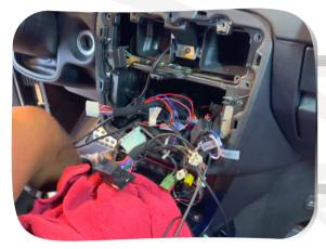
22. Unplug all the connector from the radio, and remove the radio entirely
