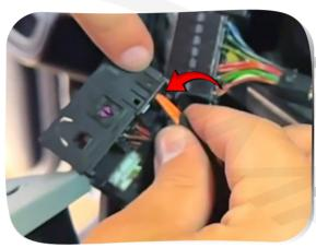
14. Transfer the fiber optic cables (Orange color) to the new harness
