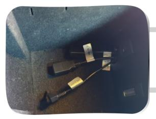
23. This step is required to route the AUX and 2 USB ports to the center storage
