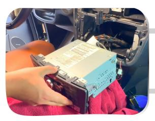
12. You can now rest the radio on the towel to gain easy acess to the connections at the back of the radio
