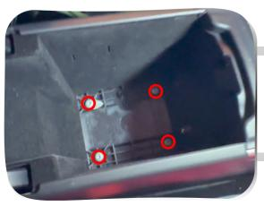
24. Remove the carpet under the center storage box and remove the 4 screws
