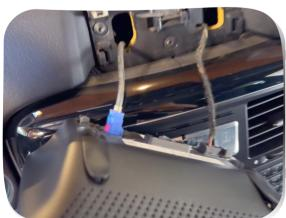
4. Unplug this 2 cables at the back of the screen. We will be using the blue LVDS cable later on the new screen
