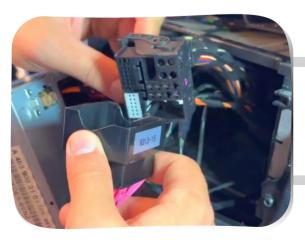
16. Plug in the original radio connector to the other end of the new harness
