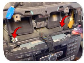
9. Remove the 2 screws under the airvent
