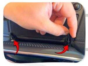
1. Pry the rubber cover on the rear of screen to expose the screws
