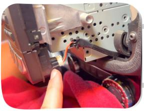
11. Remove the small connector the the bottom right of the radio
