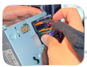
15. Plug in the new harness with the fiber optic cables into the radio
