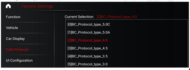
Note: If the wrong CAN protocol is selected, the display of the air conditioner on the Android screen will not work.
