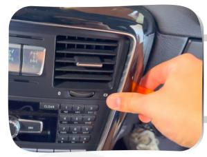
5. Use a Plastic pry too to remove the trim piece around the radio unit
