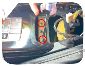
27. Remove the 2 bolts holding the shifter pannel
