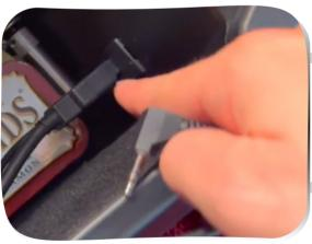
19. Connect the AUX cable inside the center storage box with an adaptor which is included with your kit
